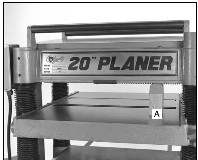
Figure 8. Measurement block in place.
